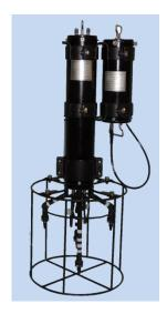
This system has been using for Monitoring and record the sound of marine mammals. Sound
